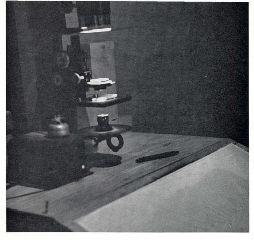
A microprojector is used to study scales. The slide is placed on the projector above and is enlarged greatly on the screen below.
